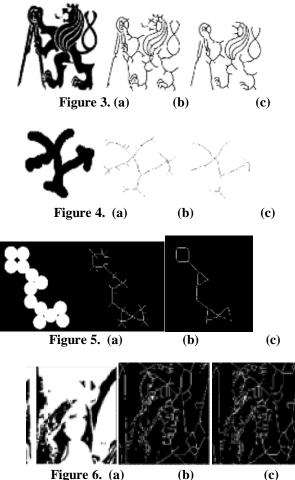
Figure 3(a), 4(a), 5(a), 6(a) - original binary images. Figure 3(b), 4(b), 5(b), 6(b) - thinned results. Figure 3(c), 4(c), 5(c), 6(c) - skeletonization results respectively.
